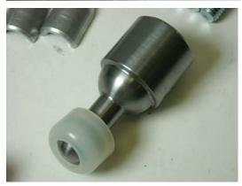
a. Slide the extension over the end of the transfer case shifter so the flat sides of the shifter are in line with the flat sides of the extension.
